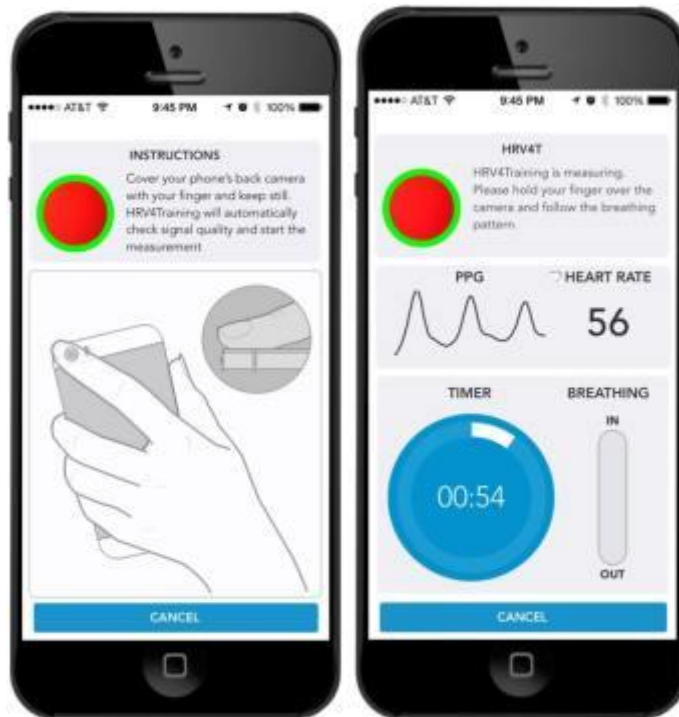
The HRV4 Training app uses your phone's camera and flash to measure heart rate
